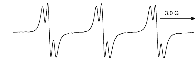
Fig. 3. EPR spectrum of PINO obtained by mixing NHPI with m -CPBA in CH 3 CN at room temperature.
